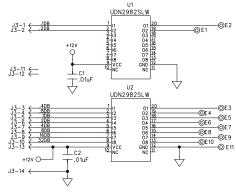
Schematic for TTL Driver Board (Option -2) with 15 pin D Connector (P/N 101-1798-000 & 101-1798-001):
